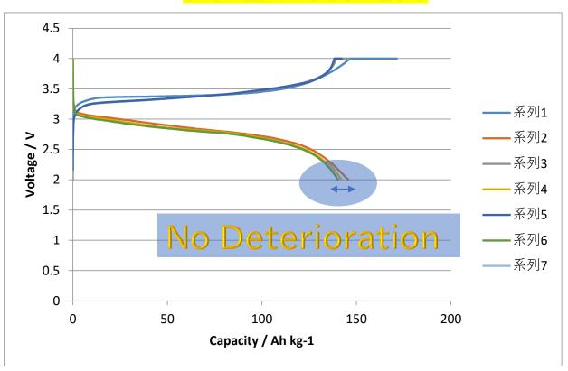
High charging/discharging efficiency from the beginning. Capacity does not decrease even after repeated use.
